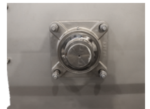
View of the silo discharge screw bearing with and without safety cover.
