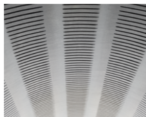
Slit filter seen from inside.
