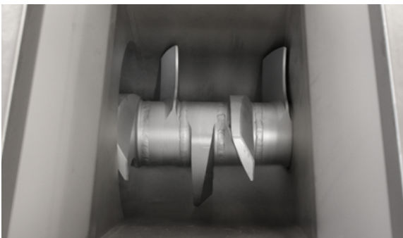
scansteel foodtech ® scanStructor top view, showing the infeed hopper with heavy duty crushing claws.
