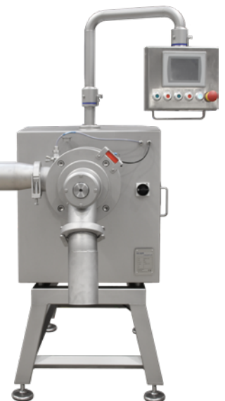
Superpump SP 250 shown below feeding a scanDebone 150.
