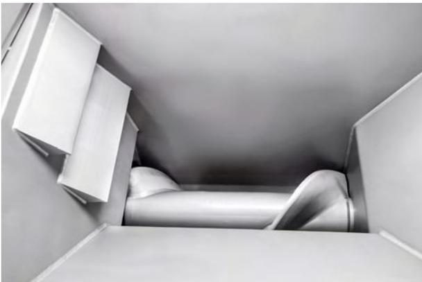
*Fresh soft meats as well as tempered or hard frozen blocks are efficiently processed jointly or separately without changing any mechanical components due to the ingenious design of hopper, transfer area between the worms/augers combined with efficient fixation of the frozen blocks. Narrow tolerances eliminate backwash, fines, or smearing.*
