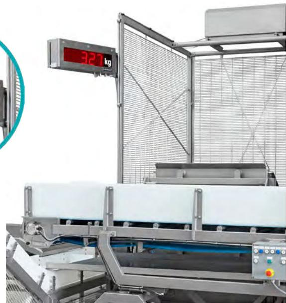
Details showing drip trays and weighing/load cells.
