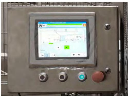
Line control of weighing and batching station.
