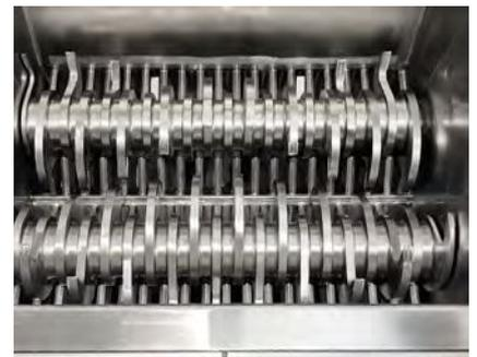
Top view looking at the inside/infeed section where the whole pallets of meat raw material will be fed into the WPC 2000.
