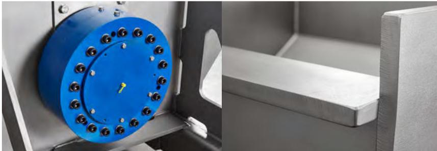
Heavy Duty bearings – on each end of the crusher claw(s). Absorbing/eliminating all axial forces between claw(s) and gear box.
