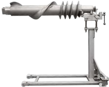
Cleaning trolley for worm/auger shown after the worm/auger has been removed from grinder.
