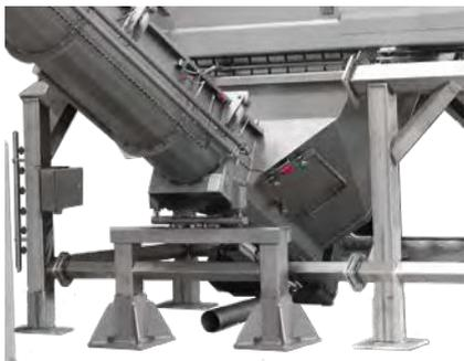
Buffer hopper with mounted weighing cells for batch control and automatic start/stop of machinery.
