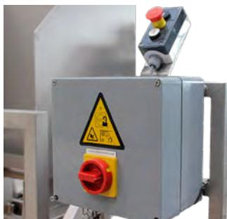
Operator/control panel with emergency stop.
