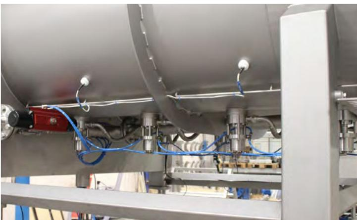
Close up of scansteel foodtech® Bottom steam injection system shown on Twin Shaft Mixer, TSM(V)
