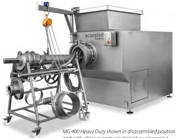
MG 400 Heavy Duty shown in disassembled position and with all loose parts positioned on accessory/ cleaning trolley for inspection and cleaning prior to assembly.
