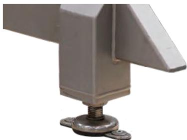
Machine feet which can be mounted to the floor.
