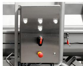
Standard screw conveyor electrical/operator panel.
