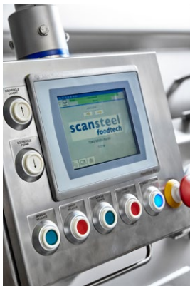
Electrical cabinets/operating panels, Allen Bradley or Siemens as standard.
