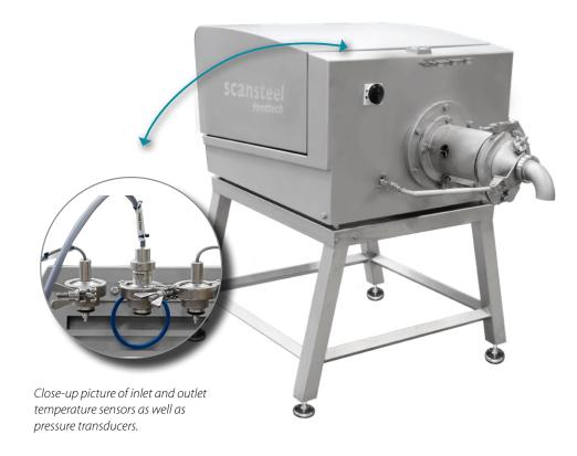
The scanEmul 175 shown below with a scansteel foodtech® ContiPump 250 with Twin Screw to avoid bridge building. Typically, the ContiPump 250 is positioned so either one or two mixers can discharge into the infeed hopper of the ContiPump 250.
