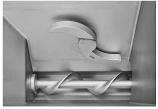
Stirring/feeding device. To secure continuous infeed of difficult/ sticky meat raw material at the grinder worm/auger.
