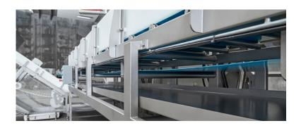
All scansteel foodtech® belt conveyors can upon customers request be manufactured with drip trays/ collection pans in order to avoid moisture on the floor.
