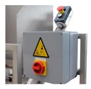
Operator/control panel with emergency stop.
