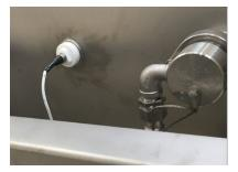
Valve shown mounted on mixer. Temperature sensor shown to the left and valve shown to the right.
