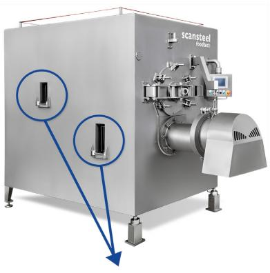
Top picture: Details of the two unique hygienic zones for both top/feeding worm and bottom/grinding worm. This unique feature physically prevents cross contamination. Protected by safety grill and safety switch, which will stop the motor in three to four seconds from activation to full stop.
