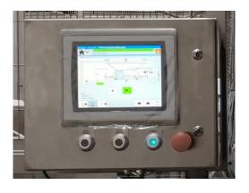
Line control of weighing and batching station.
