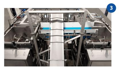
Close-up view showing scansteel foodtech® inclined screw conveyor feeding onto a scansteel foodtech® horizontal belt conveyor which has 3 (three) main positions.
