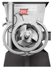
Front end of SuperGrind 400/260 shown disassembled, with worm/auger in place, ready for mounting of 3-bladed cut-knife. Cut-knife recessed into the worm/auger.
