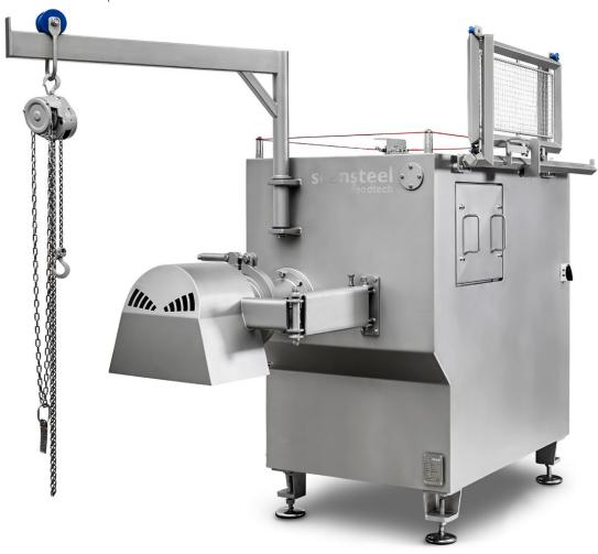
Infeed hopper secured by trip wire. When safety devices have been triggered, they will stop the machine after maximum of 4 (four) seconds.
