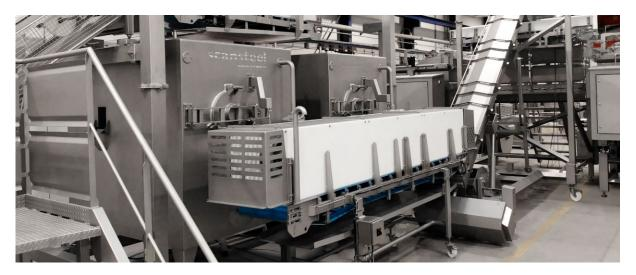
Another typical horizontal belt conveyor solution where 2 (two) grinders are discharging onto the scansteel foodtech® belt conveyor. This solution saves a lot of safety devices and, at the same time, secures easy access to the grinders for cleaning, mounting, and dismounting of the grinders, front view.
