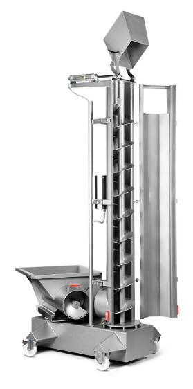
scansteel foodtech® standard scanGiraff shown in cleaning position. Note the vertical screw is 100% accessible for cleaning (no hidden zones).
