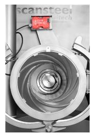
Cabinet without worm/auger showing the flights of the lining.
