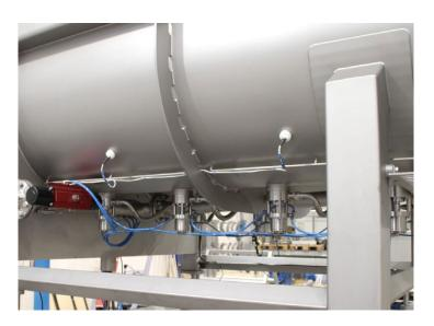
Close up of scansteel foodtech $^\circ$  Bottom steam injection system shown on Twin Shaft Mixer, TSM(V)
