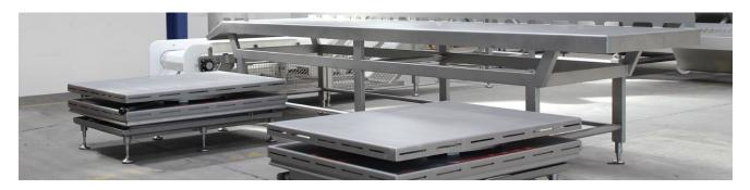
Belt Conveyor with Unpacking station with 2 (two) lifting tables for ergonomics, right side.
