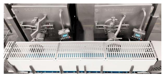
Another typical horizontal belt conveyor solution where two grinders are discharging onto the scansteel foodtech® belt conveyor. This solution saves a lot of safety devices and, at the same time, secures easy access to the grinders for cleaning, mounting and dismounting of the grinders, top view where the transfer point from grinders to belt conveyor is clearly seen.
