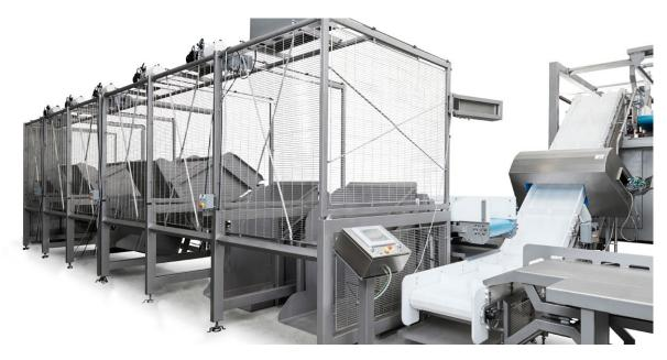
6 (six) unit weighing station, seen from the infeed side. Typically, Dolav bins are fed into the swing loaders by a fork lift truck. All is controllable from the operator panel.
