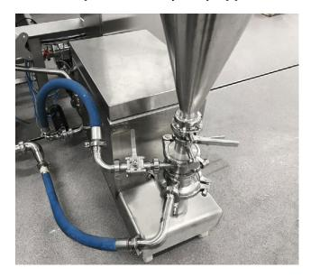
The mixing tank is used to dissolve or disperse powdered products in a liquid or to mix different liquids, with the Ytron powder dispenser for dissolving all dry "challenging to add" matters/ingredients in the gravy and/or the brine.
