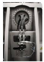
Pallet inverter seen from behind without cover, turning device.
